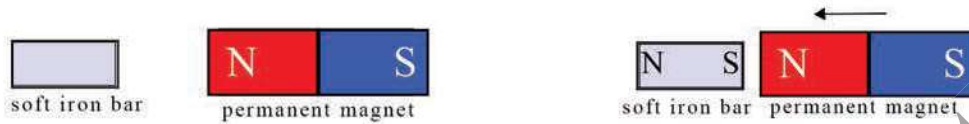
Figure 10.10 Permanent magnet brought near to soft-iron bar and soft-iron bar becomes an induced magnet
