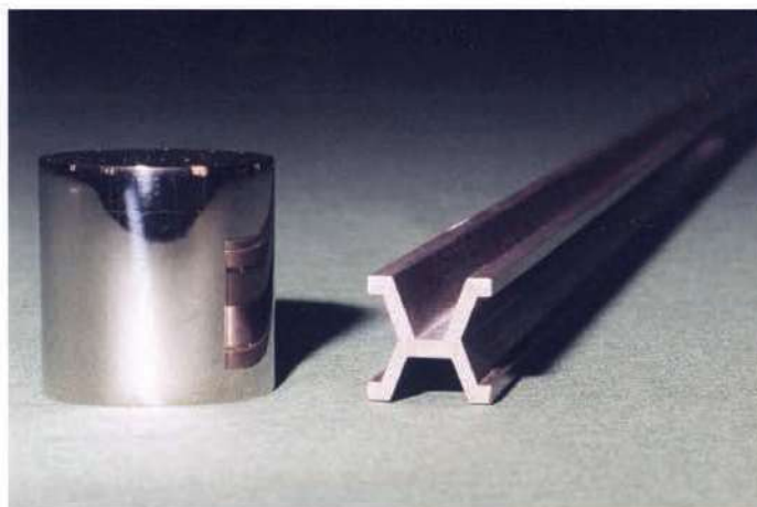
Figure 1.1 The standard kilogram and the standard metre kept at International Bureau of Weights and Measures
